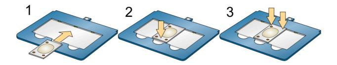
carrier. The correct slide insertion sequence is illustrated. Once the slide, or slides, are inserted, the carrier plate can be slid into place on the stage. Be sure that the carrier is securely fitted into the caliper and that the magnetic catch has engaged. You are now ready to begin observation and image capture.
